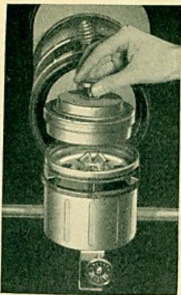
Removing Flame Spreader
