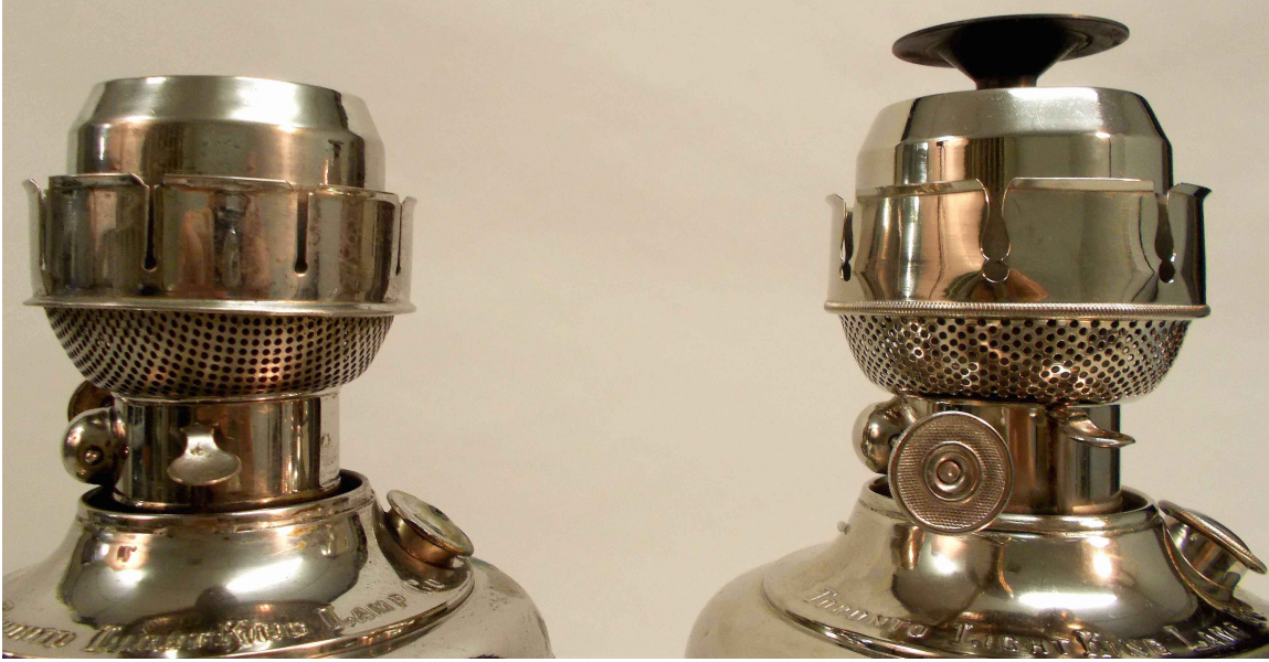
Fig. 19 - Two different gallery designs found on Toronto Light King lamps. The one on the left is from the Wellington County Museum lamp and has the same gallery pattern as the Holmes, Booth and Hayden Star Lamp shown in Figure 21. The one on the right is from the collection of the author and appears to be the same as the Bristol Electric lamp seen in Figure 18. Note the difference in the ventilation hole pattern as well as the slots in the crown. Photo P.C. Brickell.
