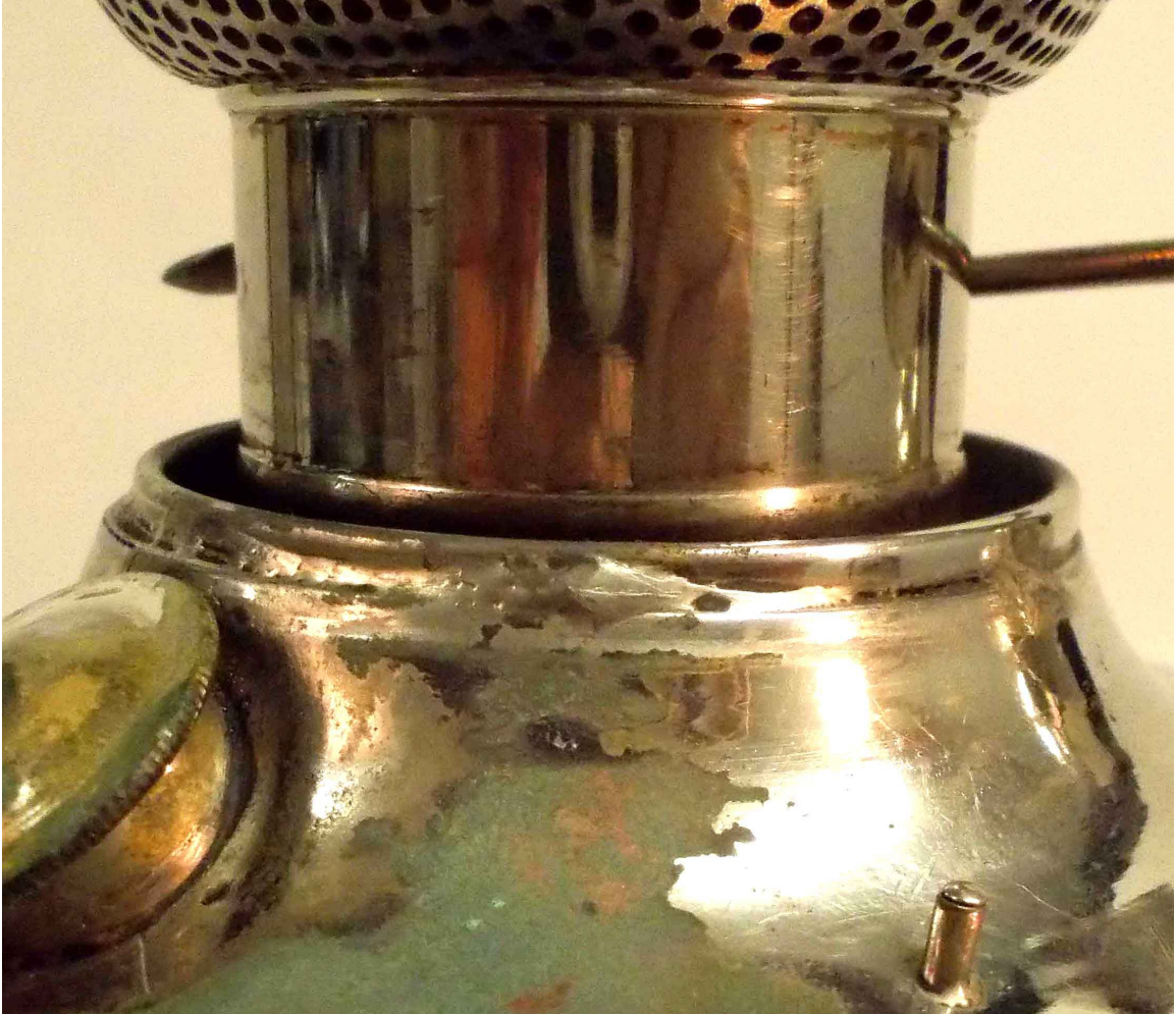
Fig.6 – Detail of air gap between the burner outer wick tube and the font. Collection of Wellington County Museum. Photo P.C. Brickell.
