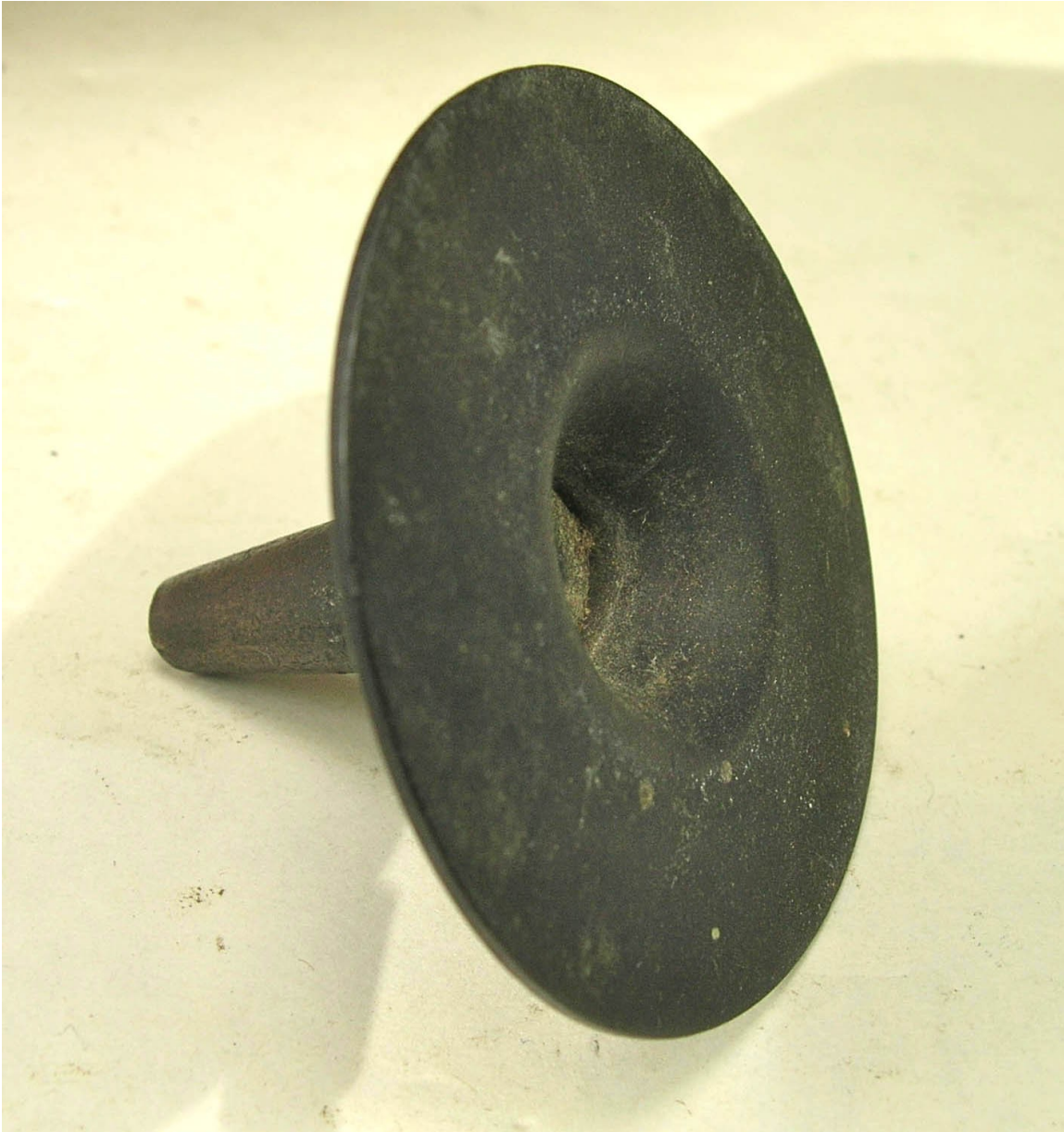
Fig.4 – Flame spreader from Holmes, Booth and Hayden “Star” lamp which is thought to be identical to that used in the Toronto Light King. Collection of Dickson Stauffer III. Photo by D. Stauffer.
