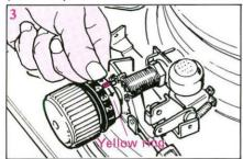
(4) Pull and turn the black ring to the right one numerical setting holding the yellow ring in position with the left hand. (Picture 4)
