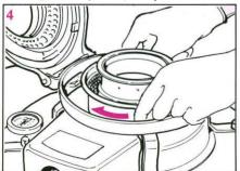
\* When replacing the wick cylinder, turn it clockwise. Line up the red marks on the wick cylinder and tank as closely as possible while making sure the wick cylinder is securely in place. (Picture 5)
