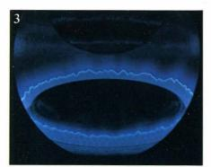
(3) CAUTION: The above setting looks normal but the flame is too low. This will cause incomplete combustion and an unpleasant odor. Adjust the flame until a flame length of at least 1 cm is obtained as indicated in Picture 1.
