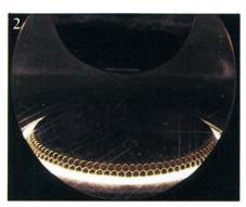
(2) The picture (2) above shows the flame just after lighting. This flame is too low. Operating the heater at this setting will result in damage to the wick, an unpleasant odor, and potentially harmful combustion by-products.
