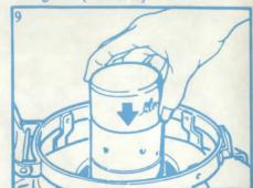
1) Release the emergency shut-off device (4) Unscrew and remove wick cylinder. (7) Remove wick and wick holder from (11) Fit skirts of new wick over wick-set- (13) Pull wick control knob and black ring guide and engage wick winder gear to rack of wick holder. (Picture 10, 11)
