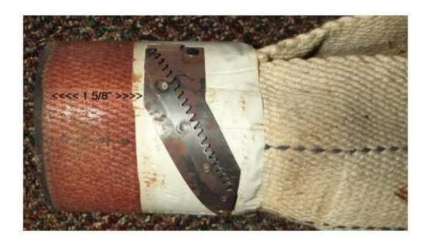
The C-10/C-20 wick was a precursor to the Aladdin Blue Flame wick now used. It is essentially the same wick, 3" diameter, cardboard lined on the inside, but had the unusual gear rack attachment as shown.
