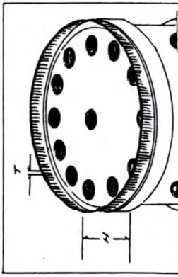
When a new wick is replaced, adjust the wick height to 6-7 mm high. The wick guide tube and (draft tube must form a concentric circle, avoid them from eccentric, otherwise the wick movement will not be smooth. Assembling procedures are progressively in reverse order described above.
