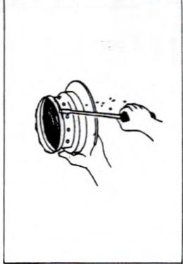
First remove a nut on the gear and the gear itself, next remove the old wick.
