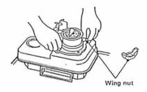
3 Remove the two set-screws situated at the right and left side of the cabinet, and then lift the cabinet upwards to remove it.
