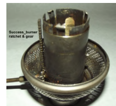
Slot in the gallery fits over peg opposite winder gear.
