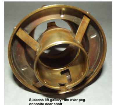
Slot in the gallery fits over peg opposite winder gear.
