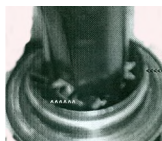
The barbs ^^^ at the end of the fingers bent to 90°.
