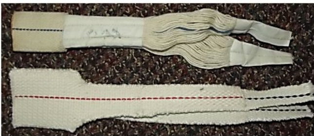
Left: Comparison: original 14" above, new hand-made 18" wick below.
